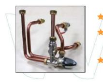
Compact solution that integrates the mixing and diverter valve According to the temperature of the water coming from the solar cylinder, water is diverted to the boiler or directly to the use Increased level of comfort and gas consumption reduction
